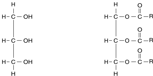
FIGURE 3.1 Chemical structure of glycerol and the chemical structure of a medium-chain triglyceride where the R represents a medium-length fatty acid.
